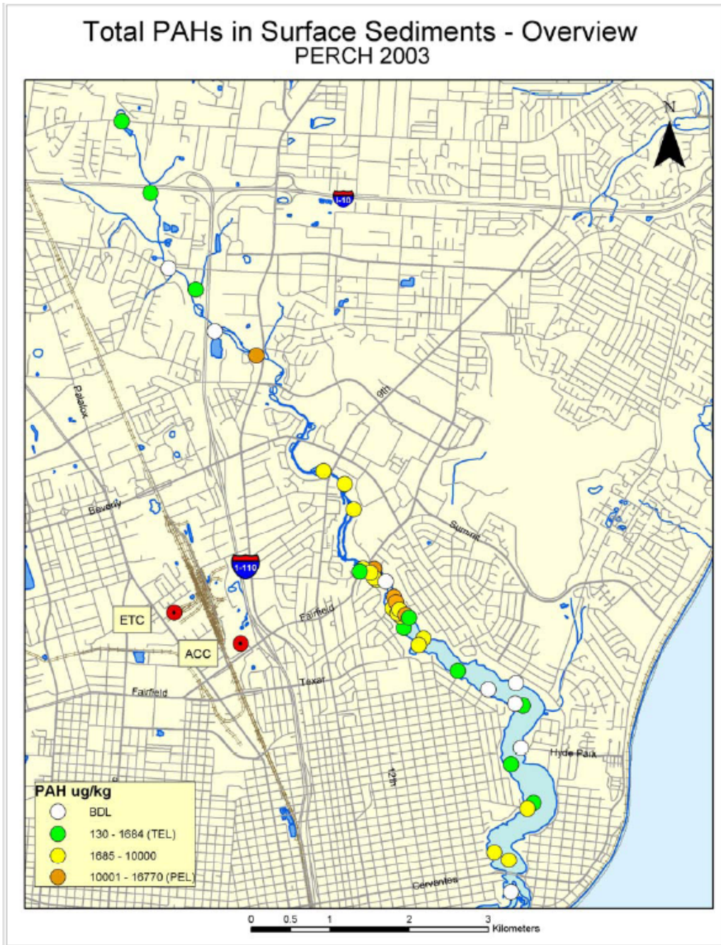
Fig. E-6. Spatial distribution of PAHs in surface sediments in Bayou Texar and Carpenter's Creek.
